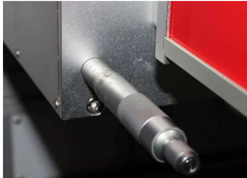
dynamic focusing head easy adjustment system
